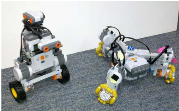
Lego robots: “Legway” inverted pendulum, 3-wheeled omni-directional robot, edge-balancing suitcase, and acrobat.
