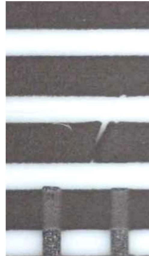
Actual photo of a missing-material defect http://www.midasvision.com/v3.htm
