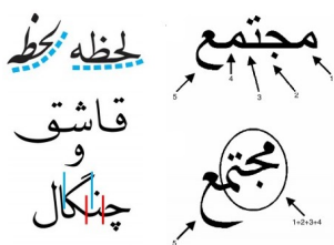
Fig. 4. For printing with movable type, the Persian script had to be made horizontally decomposable (uncredited Web images).
