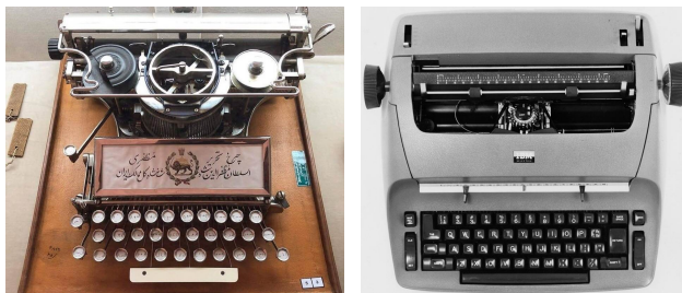
Fig. 8. Mozaffar al-Din Shah’s custom-made typewriter, ca. 1900 (Golestan Palace Museum, Tehran) and a later-model IBM Selectric with golf-ball printing mechanism, ca. 1975 (IBM).
