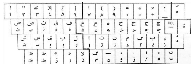
Fig. 11. Unified Persian keyboard layout, a standard for computers, typewriters, and other data-entry systems [15].
