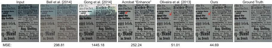
Fig. 2. We show an example from a controlled environment used to validate the correctness of our approach relative to the ground truth. We also provide the results and MSE scores of related approaches for comparison. In general, our output has minimal artifacts and is closest to ground truth in terms of average and median MSE (Table 1). See the supplemental materials for additional results from this controlled setting.
