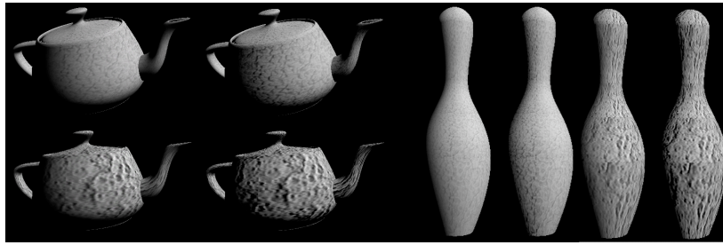
Figure 2: Screen shots of a real-time hardware implementation of our approach, using the Gaussian random texture (the 10^\circ sample) from Figure 3 and a plaster texture from the Curet database. For every object, we show it rendered using conventional 2D texture mapping on the left, and our 2\frac{1}{2} D texture mapping on the right. The images render at over 100 fps and the objects can be rotated interactively.
