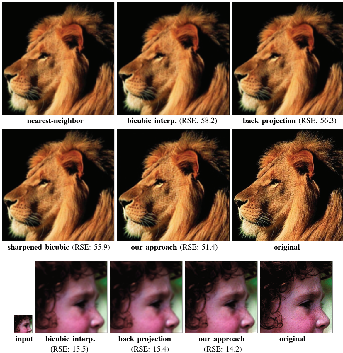
Fig. 1. These two images have been magnified by a factor of 4 and the results of various standard algorithms are compared. The proposed algorithm produces an upsampled image with more detail and lower RSE than the other approaches.
