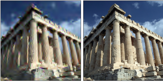
Fig. 4. The problem of not using the Gaussian filter formulation. On the left, we show the result of simply point-sampling the initial image to downsample by a factor of 2 and then reconstructing by solving the CS problem using wavelet compression but without the blurring filter \Phi (RSE: 85.5). The result is unusable because the coherency between the point-samples and the wavelet basis breaks down the CS approach. On the right, we use our proposed formulation with a blur filter and the image quality is significantly improved (RSE: 40.6). For comparison, the RSE for bicubic interpolation is 51.9.
