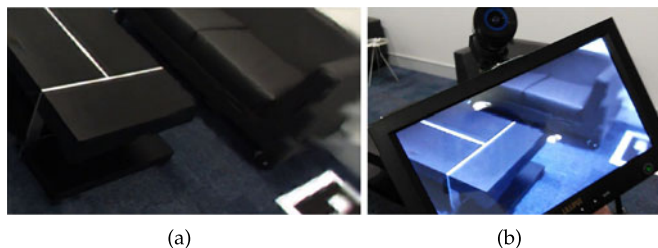
Fig. 11. Synchronized (a) screen capture and (b) and user view, showing artifacts that can occur due to failure cases. These include streaks/breaks caused by disparity errors, and blurriness at the edge of the observed scene. (Note: the bright spots on the screen are reflections of the room lights.)
