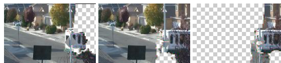
Figure 7: Visualizing removed pixels. Each frame above has pixels removed. Although pixels are removed from multiple frames, the total length of the video is reduced by 1 frame.
