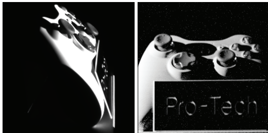
Figure 3: An example of a primal-dual pair, with the primal image on the left and the dual on the right. One of the surprising things about dual photography is how certain detail can be drastically enhanced in the dual image. For example, the “Pro-Tech” text is unreadable in the primal image, yet clearly visible in the dual (see electronic version of this paper for clear reproduction). It is almost surprising that we would be able to reconstruct this text using only images like those on the left. The images have a resolution of 256 \times 256 and were captured using 1,500 patterns.
