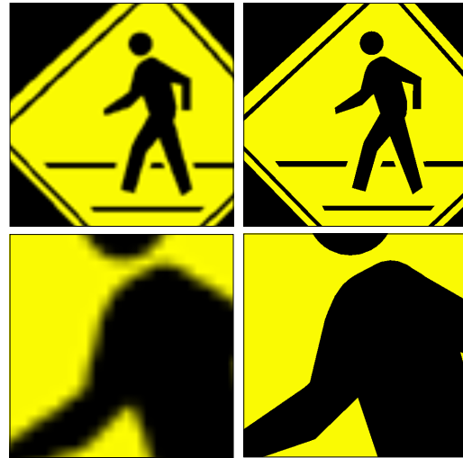
Figure 8: An example of a sign that might appear in a racing video game, with resolution 128 \times 128 . The parts shown are magnified to 512 \times 512 . (Left) Standard texturing with bilinear interpolation. (Right) Our technique.
