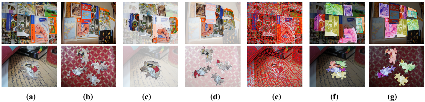
Fig. 12. Results of unsupervised co-recognition using our algorithm. The first line shows the BOOKS example, and the second line shows the JIGSAW example. (a) Source images. (b) Reference images. (c) Source images highlighted with NRDC correspondences. (d) Reference images highlighted with NRDC correspondences. (e) Source image segmentation. (f) Objects detected in source images by our algorithm. (g) Objects detected in reference images by our algorithm. Different objects are masked with different colors. Our method recognizes most parts of shared objects accurately.
