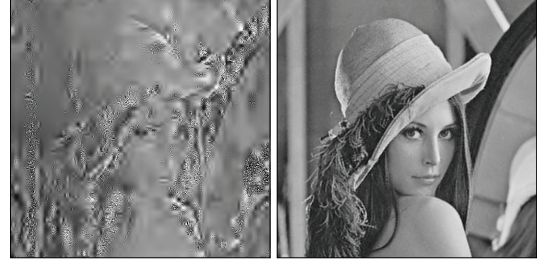
Fig. 2. (left) CS reconstruction with wavelets from 25% pixel samples has problems since \Psi is not incoherent with point-sampled \mathbf{S} (PSNR = 13.4dB). (right) Result of using the filtered wavelet formulation presented from the same samples (PSNR = 32.7dB). This new approach beats traditional interpolation techniques.
