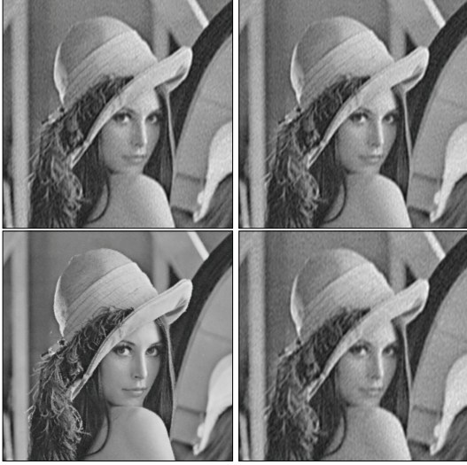
Fig. 1. CS imaging with Fourier basis. The top row shows the results of using a sparsified version of the LENA image. On the left is the input, where all but the 2% largest Fourier coefficients have been forced to zero. On the right is the reconstruction using CS from 25% of pixels samples. The two are virtually identical (PSNR = 87.8dB). On the bottom row , we show the problem with using this approach on real images. On the left we reconstruct the original Lena image using simple interpolation from 25% of the pixels (PSNR = 32.2dB). On the right, we reconstruct from the same samples using CS and a Fourier basis (PSNR = 27.4dB). These results were initially discouraging, since CS is easily beat by the far simpler interpolation.
