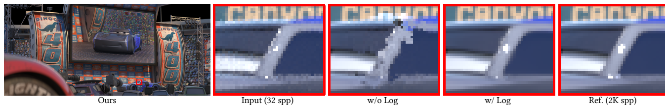
Fig. 12. When we train with high dynamic range images, we observe artifacts in regions with large-valued specular highlights. Our full approach with the log and corresponding transformed variance handles these difficult cases better.
