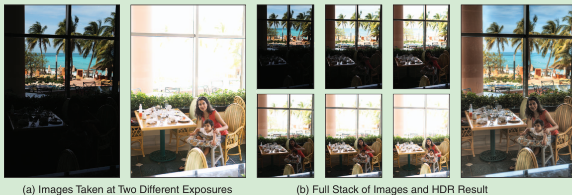
FIGURE 1. (a) Images captured by standard digital cameras cannot reproduce the wide range of illumination we see in everyday scenes, even after adjusting the exposure, as illustrated by these two images taken at different exposures. (b) HDR imaging allows for the capture of a wider range of illumination; here, a stack of images was captured at different exposures (left) and merged with the algorithm described in [1] to reduce motion artifacts and produce the result shown on the right.
