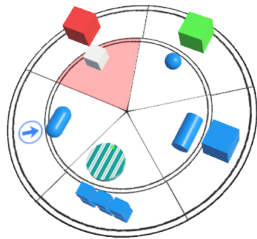
Figure 4: Our pie menu with some 3D geometry to showcase the functionality of each control. The menu appears above the touchpad on the controller.
