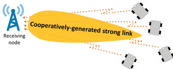
Figure 8: Distributed robotic transmit beamforming: Multiple robots cooperatively generate a strong communication link to the remote station by optimizing their locations. Figure adapted from (45).
