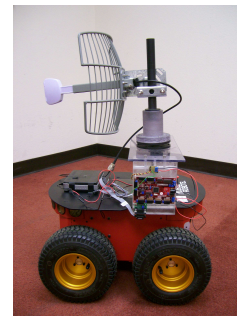
Fig. 5. Our robotic platform – Pioneer 3-AT robot equipped with a servo control mechanism/fixture and a directional antenna.
