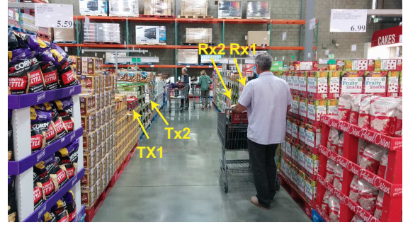
Fig. 14: The Costco experiment – the figure shows the considered “snacks and cookies” aisle in Costco along with a pair of WiFi links positioned along the aisle to make wireless measurements.
