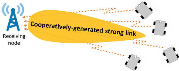
Fig. 1: Distributed robotic transmit beamforming. The robots can cooperatively generate a strong communication link by optimizing their locations.
