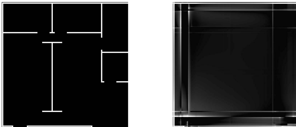
Fig. 9. Reconstruction of the map of Fig. 6 (left) with (left) our proposed approach and (right) interpolation. 11.7 percent measurements are used for both cases and no multipath fading is simulated. It can be seen that interpolation results in a considerable performance degradation.
