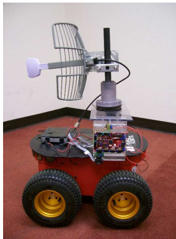
Fig. 2. The figure shows a Pioneer 3-AT robot with the additionally-mounted servomechanism and a directional antenna.
