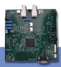
**AutoPonix** is an automated water quality monitor and adjustment system for the maintenance of an aquaponics system. The pH, temperature and conductivity of the water are all monitored, controlled and logged. The data are transmitted via WiFi to a server that hosts a site displaying charts of system data.
