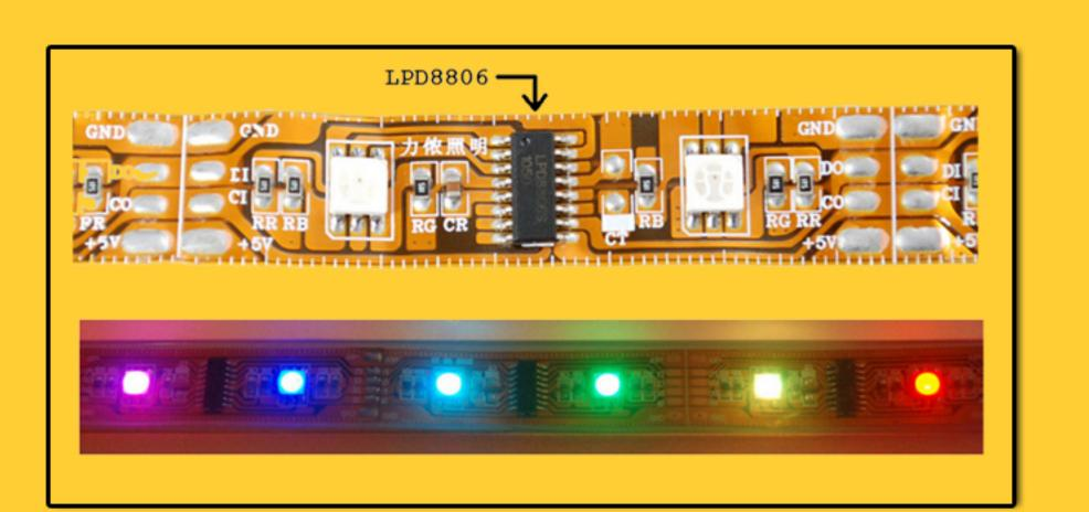
A digital RGB-LED strip is driven via the on-board SSP interface, in order to illuminate the valid moves each player can make for a specific piece they have chosen. Blue and green lights are used to represent player-specific moves, while red is displayed beneath a piece that can be taken.
