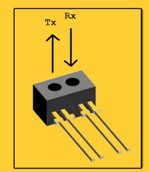
Vishay TCRT1010 proximity infrared sensors are used to detect physical piece movement, which is used in computing valid moves & tracking the game's state.
