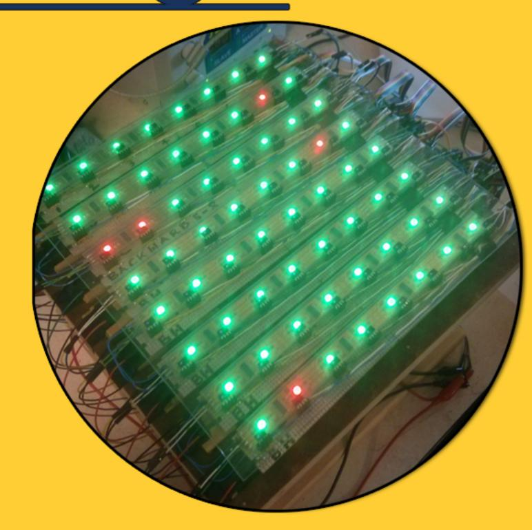
The board enclosure houses an IR sensor beneath each game tile. A digital LED lays beneath each sensor, illuminating the playing surface where desired. The sensors & LEDs communicate with the PCB, which sits at the very bottom of the enclosure.
