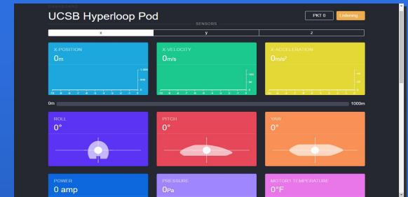
Figure 9: Hyperloop Web App Monitors Position, Power, Temperature
