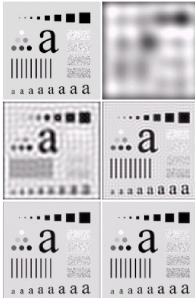
FIGURE 4.12 (a) Original image. (b)–(f) Results of ideal lowpass filtering with cutoff frequencies set at radii values of 5, 15, 30, 80, and 230, as shown in Fig. 4.11(b). The power removed by these filters was 8, 5.4, 3.6, 2, and 0.5% of the total, respectively.
