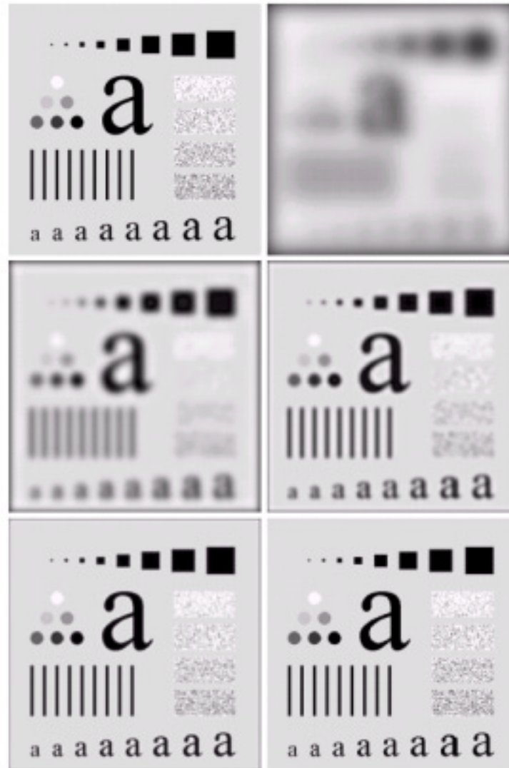
FIGURE 4.15 (a) Original image. (b)–(f) Results of filtering with BLPFs of order 2, with cutoff frequencies at radii of 5, 15, 30, 80, and 230, as shown in Fig. 4.11(b). Compare with Fig. 4.12.
