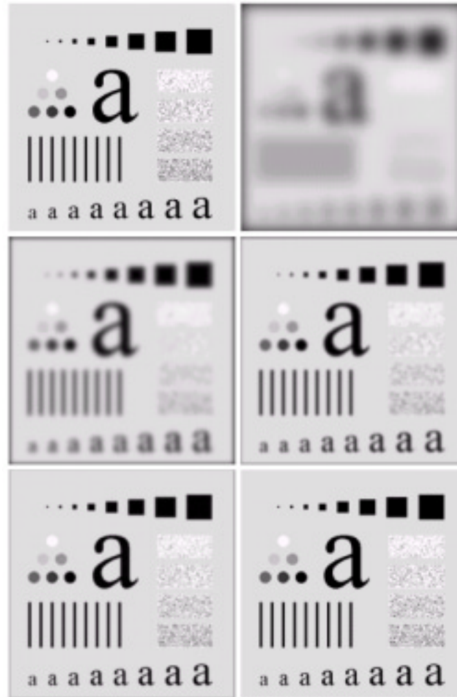
FIGURE 4.18 (a) Original image. (b)–(f) Results of filtering with Gaussian lowpass filters with cutoff frequencies set at radii values of 5, 15, 30, 80, and 230, as shown in Fig. 4.11(b). Compare with Figs. 4.12 and 4.15.
