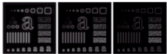
FIGURE 4.25 Results of highpass filtering the image in Fig. 4.11(a) using a BHPF of order 2 with d_0 = 15, 30, \text{ and } 90 , respectively. These results are much smoother than those obtained with an IHPF.
