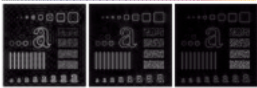
FIGURE 4.24 Results of ideal highpass filtering the image in Fig. 4.11(a) with d_0 = 15, 30, \text{ and } 90 , respectively. Problems with ringing are quite evident in (a) and (b).
