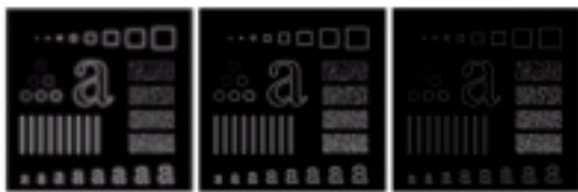
FIGURE 4.26 Results of highpass filtering the image of Fig. 4.11(a) using a GHPF of order 2 with d_0 = 15, 30, \text{ and } 90 , respectively. Compare with Figs. 4.24 and 4.25.
