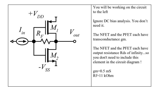
Compute, from nodal analysis, the small-signal gain Vout/Iin. This is called a transimpedance gain.
