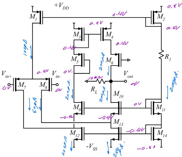
The NMOSFETs have  $K_{\mu} = \mu c_{gs} W_g / 2L_g = 10 \text{mA/V}^2 \cdot (W_g / 1\mu \text{m})$   $K_v = c_{gs} v_{inj} W_g = 2.0 \text{mA/V} \cdot (W_g / 1\mu \text{m}), \ \Delta V = v_{inj} L_g / \mu = 0.10 \text{V}, \ V_{th} = 0.3 \text{V},$  $1/\lambda = 5 \text{V}$
