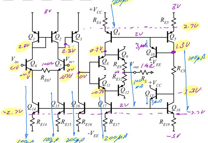
On the circuit diagram above, label the DC voltages at ALL nodes, and the DC collector currents of all transistors. Label the values of all resistors.
