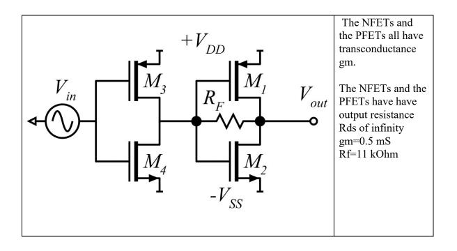
Compute, from nodal analysis, the small-signal gain Vout/Vin. This is a voltage gain. Hint: you can save some work by using the result from part A.
