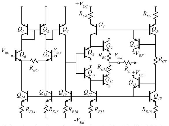
All the transistors have the same (matched)  $I_s$ , have  $\beta = 100$ , and  $V_A = *infinity*$  Volts.  $V_{CE(sat)} = 0.5$ V.  $V_{be}$  is approximately 0.7 V, but use  $V_{be} = (kT/q)\ln(I_E/I_s)$  when necessary or appropriate. The supplies are +3 Volts and -3 Volts. All transistors have the same  $I_s$ .
