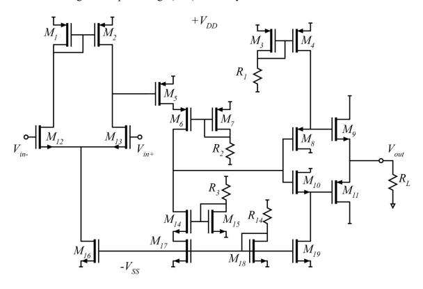
The NMOSFETs have  $K_{\mu} = \mu c_{gs} W_g / 2L_g = 0.55 \text{mA/V}^2 \cdot (W_g / 1 \mu \text{m})$
