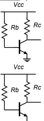
a) beta=75 Vcc=15 volts We want 0.5mA collector current, and Vce=3 Volts Find Rc and Rb
