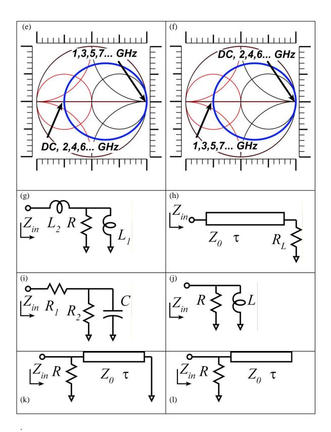
First match each Smith Chart with each circuit. *Then determine as many component values as is possible* (RLC values, transmission line delays and characteristic impedances)...note that some values cannot be determined with the information given. The charts all use 50 Ohm normalization:
