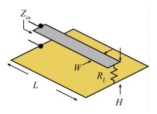
Part c, 10 points If the line is loaded by RL=1 Ohms, find the value for Zin at 2.5GHz signal frequency.
