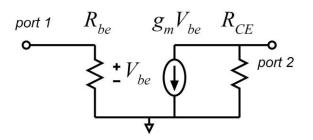
Part b, 15 points First, compute S11 and S21, both as a function of frequency, for this network.
