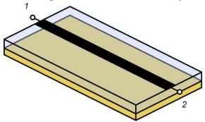
We will make a 50 Ohm microstrip line on commercial board material (like that used in the class) with a dielectric constant of 2.2.
