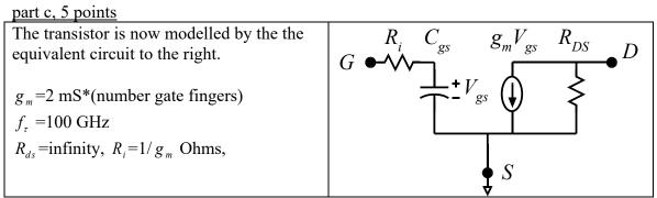
Given a 10 Ohm load, and the number of gate fingers you have found earlier, what input power at 10 GHz is necessary to produce this maximum output power ?
