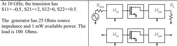
We first impedance-match the generator to the transistor input and then impedance-match the load to the transistor output (upper diagram). We then disconnect the generator and the load (lower diagram), leaving us with the transistor and its input and output networks, which we can an "amplifier".
