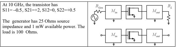
We first impedance-match the generator to the transistor input and then impedance-match the load to the transistor output (upper diagram). We then disconnect the generator and the load (lower diagram), leaving us with the transistor and its input and output networks, which we can an "amplifier".
