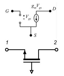
Now, given this model, for the network at the right, give the numerical values of S21 and S11. The reference Zo is 50 Ohms. .
