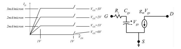
A FET has the common-source characteristics above, normalize to FET gate width. You can infer gm from the data above. We have Ri=1/gm, and  $f_{\tau}$  is 200 GHz. The signal frequency is 50 GHz
