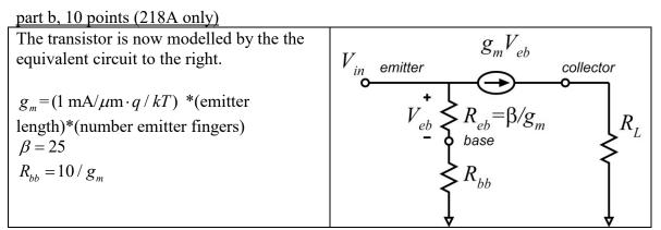
Given the 50 Ohm load, the 5 micron emitter length, and the number of emitter fingers you have found earlier, what input power is necessary to produce this maximum output power ?
