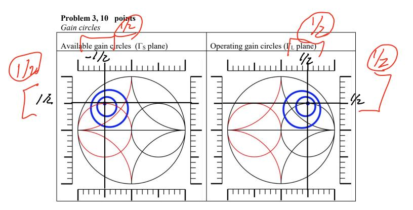
A FET in common-source mode has operating and available gain circles as shown (50 Ohm impedance normalization). Find the optimum generator and load impedances (in complex Ohms).
