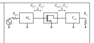
We are desinging a \*power amplifier\*. We have independently determined from  $V_{\rm max}$ ,  $V_{\min}$  ,  $I_{\max}$  , etc. , that the optimum large-signal transistor load impedance is  $Z_{L,T}$ =200  $\Omega$  and that the maximum output power, at clipping, is 100 mW. We impedance-match on metel on inpot not match on cutpat S the input.
