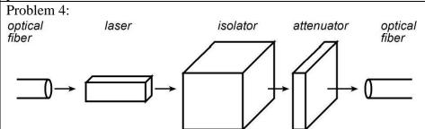
A laser (more precisely, a semiconductor optical amplifier) is coupled to an isolator and an attenuator to help stabilize it. Defining port 1 on the left and port 2 on the right, we have
