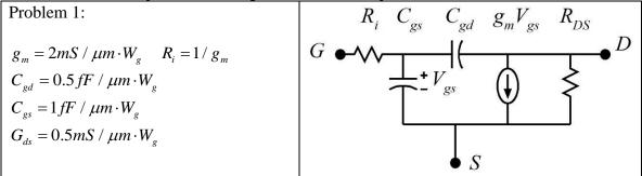
part a) Taking  $W_{p} = 50$  microns for the bilateral device model, Plot the MAG/MSG
