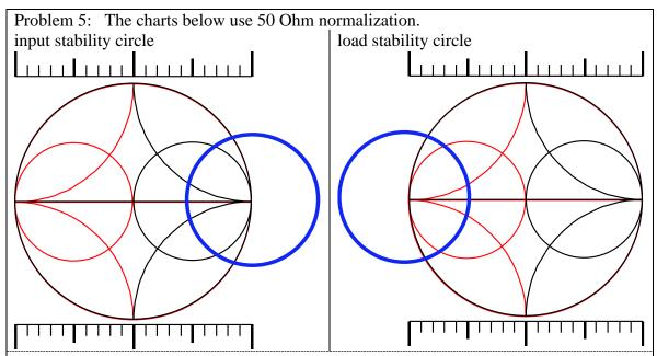
A FET in common-source configuration has the stability circles as shown above at 20 GHz. The magnitudes of both S11 and S22 are less than 1. Draw (two) circuit diagrams of two (different) stabilization methods for the transistor, giving required numerical element values. Use the scales above, along with a straight edge (edge of paper, a calculator, a book..) to aid you.
