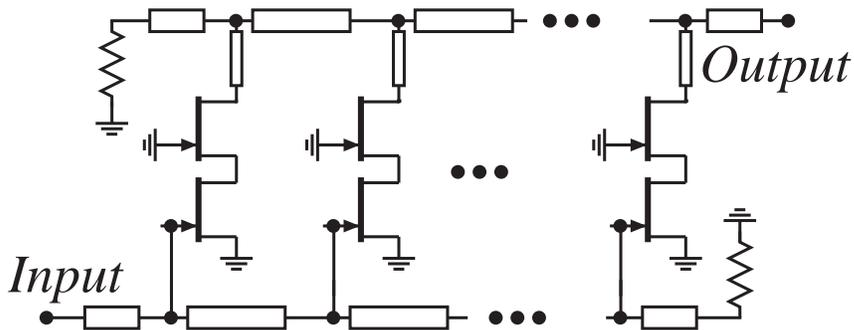
Circuit diagrams of a cascode traveling wave amplifier are shown on the previous page. As illustrated in b-c, a cascode combination can be viewed approximately as a single fet, where  $R_i$ ,  $g_m$ ,  $C_{gs}$  are unchanged, and  $R_{out}$  is many times  $R_{ds}$ . We will neglect the capacitance  $C_{out}$ .
