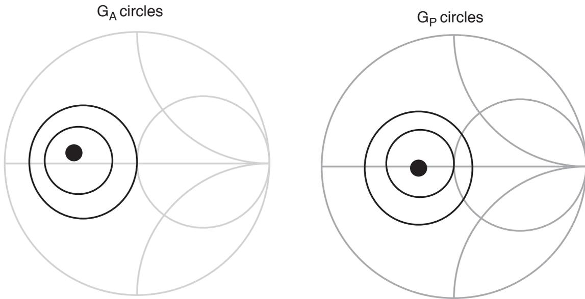
Here are  $G_A$  and  $G_P$  circles for a transistor, at 1 dB increments in Gain ( $50\Omega$  impedance standard for the impedance charts). The transistor maximum available gain is 10 dB. If the input is impedance matched to the transistor, but the load impedance is  $50\Omega$ , what is the transistor transducer power gain?
