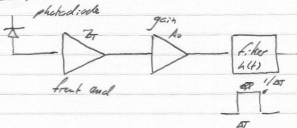
Here is an optical receiver. Photocurrent is amplified and then filtered ( $h(t)$ ) over a time  $\Delta T \sim 1/\text{Bit rate}$ . The bit rate is 40 Gb/sec, and the photodiode has ~~100 nA~~ <sup>100 nA</sup> leakage.
