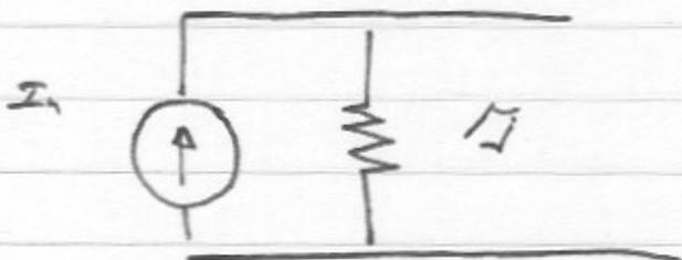
$$\frac{\partial \langle I_1 I_1^* \rangle}{\partial t} = 2gI, \quad r_j = \frac{kT}{qI}$$
