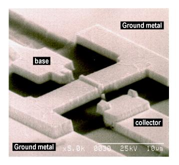
Figure 3.6: Old device interconnect scheme showing tall Metal-1 step-coverage
