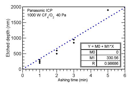
Figure B.1: BCB etch rate for the given  $CF_4/O_2$  recipe
