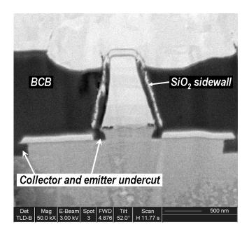
Figure 3.21: Cross-sectional SEM of an mHBT after passivation and device interconnect
