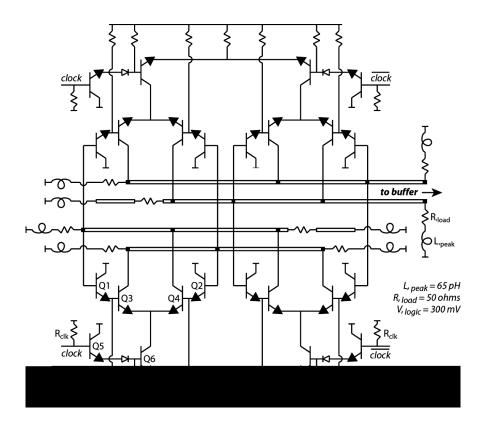
Figure 5.1: Circuit diagram of ECL static frequency divider w/ design details
