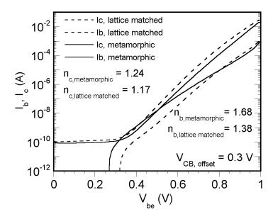
Figure 4.36: Gummel curves – comparing metamorphic and lattice-matched DHBT characteristics
