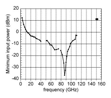
Figure 5.13: Sensitivity plot of 150 GHz divide-by-2
