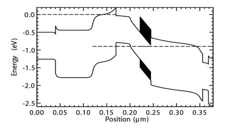
Figure 4.1: Simulated band-structure DHBT 19b –  $V_{be}$  = 0.9 V,  $V_{cb}$  = 0.0 V
