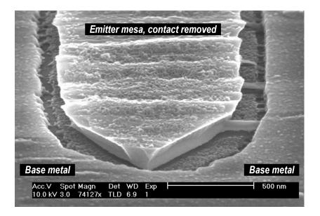
Figure 3.18: Inspection of emitter mesa after wet-etching. Note, the emitter contact has been removed
