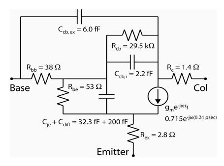
Figure 4.31: Hybrid- $\pi$  model, DHBT 27 – Peak  $f_{\tau}$ ,  $f_{max}$
