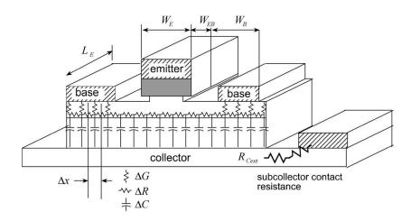
Figure 2.2: Mesa HBT showing distributed device resistances and capacitances
