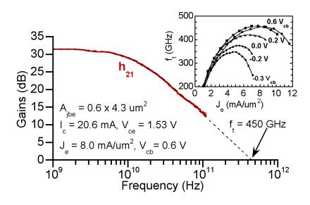
Figure 4.29: Measured microwave gains, DHBT 27 – Peak  $f_{\tau}$
