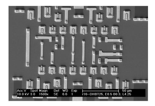
Figure 3.9: SEM of divider core before device passivation and metal interconnects
