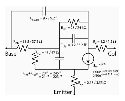
Figure 4.23: Hybrid- $\pi$  models, 100 collector, 42 / 25 nm transitions – Peak  $f_{ au},\,f_{max}$
