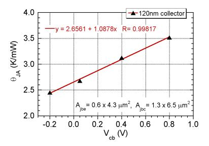
Figure 4.28: Variance of thermal resistance  $\theta_{JA}$  with changing collector potential
