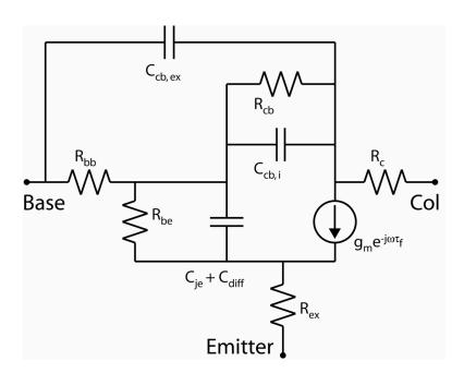
Figure 2.7: Hybrid-pi equivalent circuit HBT model
