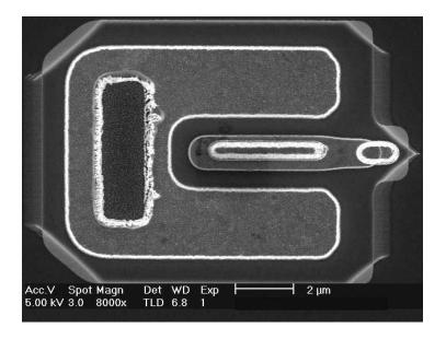
Figure 3.8: SEM, top view – 0.6  $\mu$ m emitter width, 1.3  $\mu$ m collector mesa width
