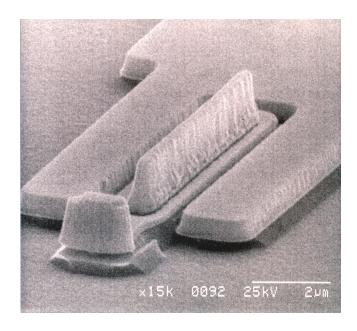
Figure 3.2: Angled SEM of an HBT before passivation
