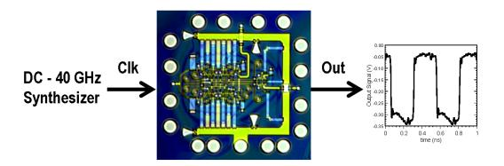
Figure 5.2: DC-40 GHz divider testing
