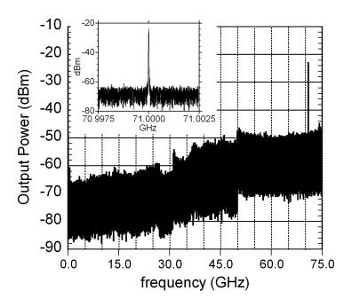
Figure 5.16: UCSB fabricated divide-by-2 output spectrum,  $f_{clk}$  = 142 GHz,  $f_{out}$  = 71 GHz
