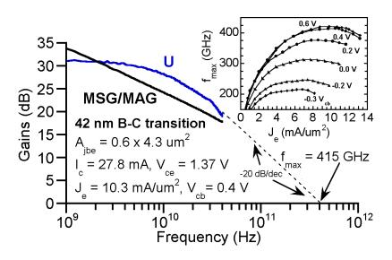
Figure 4.17: Measured microwave gains, DHBT 25 – Peak  $f_{max}$
