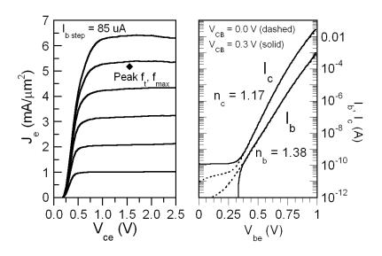
Figure 4.5: Common-emitter I-V and Gummel characteristics, DHBT 22
