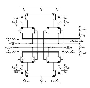
Figure 4.33: Schematic of current mode logic (CML) static frequency divider
