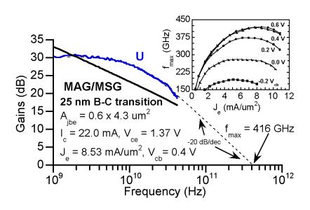
Figure 4.19: Measured microwave gains, DHBT 26 – Peak  $f_{max}$
