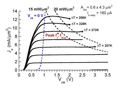
Figure 4.26: Common-emitter current-voltage characteristics, DHBT 27
