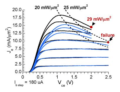
Figure 4.22: High-power density common-emitter curves – 42 nm transition (DHBT 25) black, 25 nm transition (DHBT 26) blue
