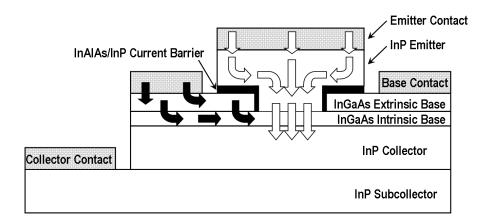
Figure 2.16: Regrown-emitter process schematic
