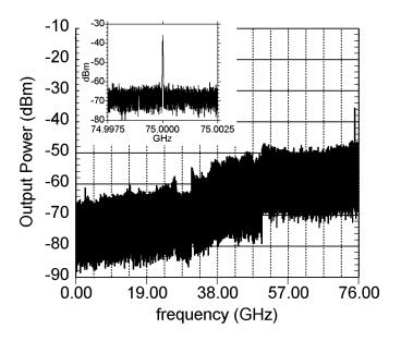
Figure 5.11: GCS fabricated divide-by-2 output spectrum,  $f_{clk}$  = 150 GHz,  $f_{out}$  = 75 GHz at T = 25°C
