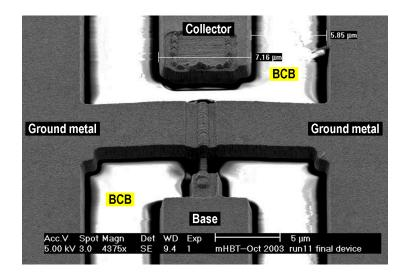
Figure 3.10: Planar device interconnect scheme: metal interconnect on 1.7  $\mu m$  of BCB above InP substrate
