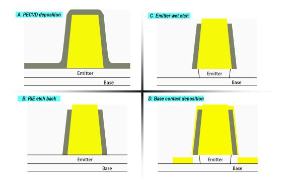
Figure 3.20: Process flow for emitter dielectric sidewall spacer
