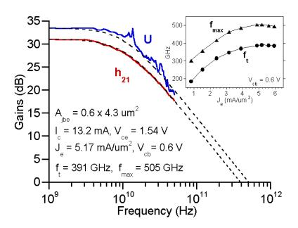
Figure 4.6: Measured microwave gains, DHBT 22 – Peak  $f_{\tau}$ ,  $f_{max}$
