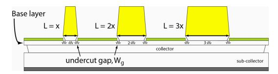
Figure 2.5: Pinched TLM structure – the emitter resides atop the base semiconductor
