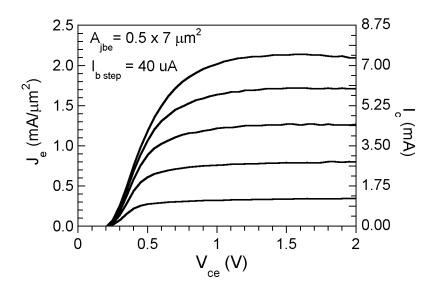
Figure 4.35: Common-emitter current-voltage characteristics, mHBT
