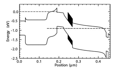
Figure 4.8: Simulated band-structure DHBT 24  $- V_{be} = 0.9 \text{ V}, V_{cb} = 0.0 \text{ V}$
