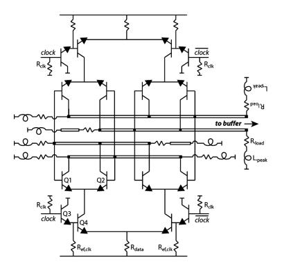
Figure 2.11: Schematic of CML static frequency divider
