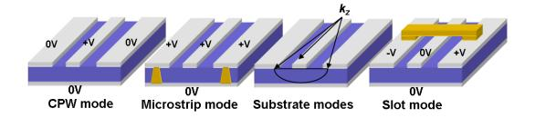
Figure 3.13: Coplanar wiring environment – showing the CPW and parasitic modes
