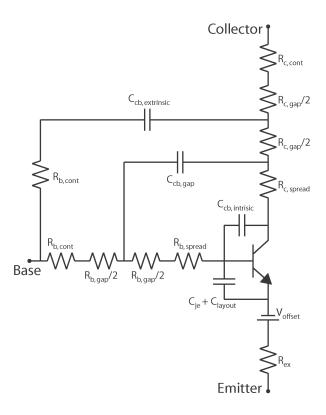
Figure 2.9: Distributed parasitics of mathematical device model
