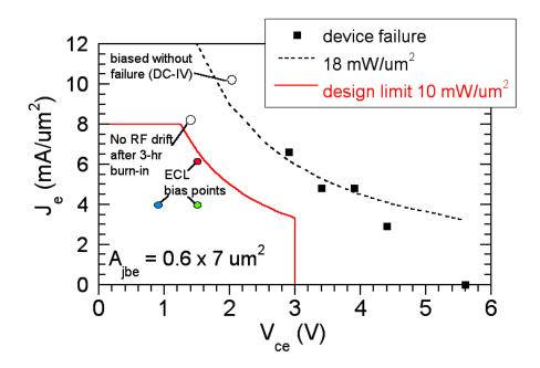
Figure 2.10: InP DHBT safe operating area plot – 150 nm collector, 30 nm base
