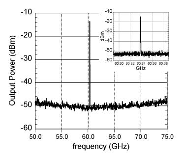
Figure 5.17: RSC fabricated divide-by-2 output spectrum,  $f_{clk}$  = 120.68 GHz,  $f_{out}$  = 60.34 GHz
