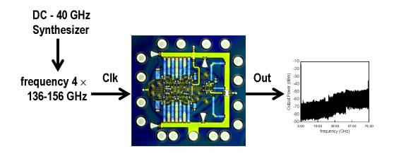
Figure 5.5: 136-156 GHz divider testing
