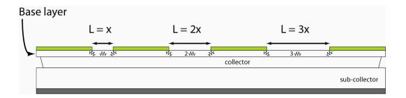
Figure 2.4: Non-pinched TLM structure – the base semiconductor is exposed
