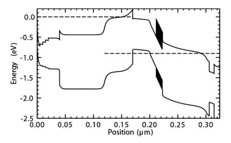
Figure 4.13: Simulated band-structure DHBT  $26 - V_{be} = 0.9 \text{ V}$ ,  $V_{cb} = 0.0 \text{ V}$
