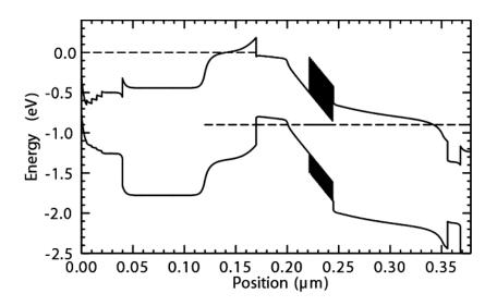
Figure 4.4: Simulated band-structure DHBT  $22 - V_{be} = 0.9 \text{ V}$ ,  $V_{cb} = 0.0 \text{ V}$
