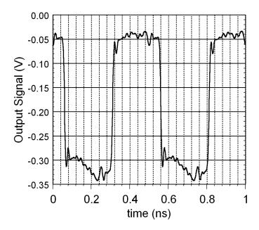
Figure 5.14: UCSB divide-by-2 output waveform,  $f_{clk} = 4$  GHz,  $f_{out} = 2$  GHz
