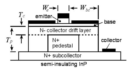
Figure 2.15: Pedestal process schematic
