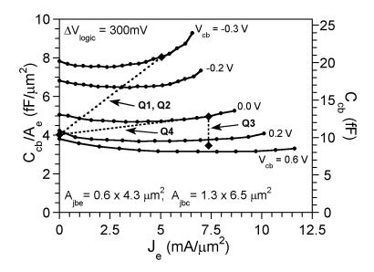
Figure 4.32: Comparison of  $C_{cb}$  vs  $J_e$  and  $V_{cb}$ , DHBT 27, labeled to show the corresponding device switching endpoints within a CML divider schematic Fig. 4.33. Lines connecting the switching endpoints have been superimposed to act as a guide.
