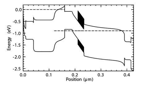
Figure 4.34: Simulated band-structure mHBT –  $V_{be}$  = 0.9 V,  $V_{cb}$  = 0.0 V
