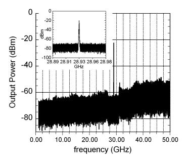
Figure 5.7: GCS fabricated divide-by-4 output spectrum,  $f_{clk}$  = 115.72 GHz,  $f_{out}$  = 28.93 GHz
