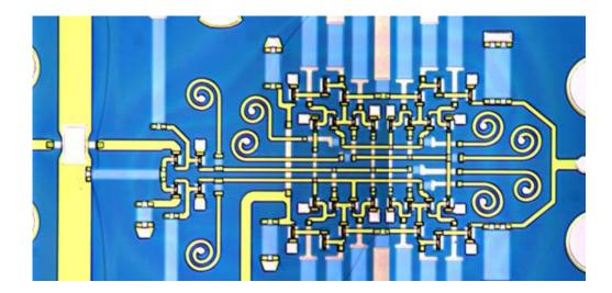
Figure 3.12: IC micrograph photo of a static frequency divider interconnect bus after Metal-1 interconnect
