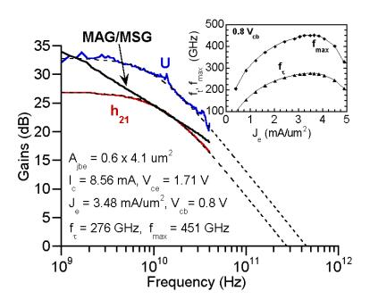
Figure 4.10: Measured microwave gains, DHBT 24 – Peak  $f_{\tau}$ ,  $f_{max}$
