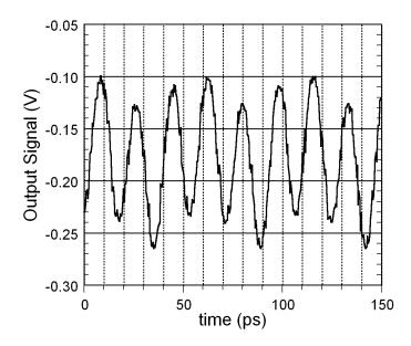
Figure 5.15: UCSB divide-by-2 output waveform,  $f_{clk} = 113.1$  GHz,  $f_{out} = 56.55$  GHz—the highest available sampling scope measurement
