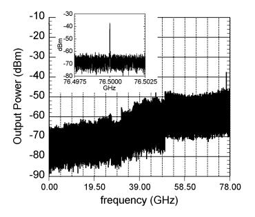
Figure 5.12: GCS fabricated divide-by-2 output spectrum,  $f_{clk}$  = 153 GHz,  $f_{out}$  = 76.5 GHz at T = 20°C
