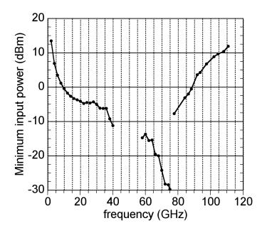
Figure 5.8: Sensitivity plot of 118.7 GHz divide-by-2
