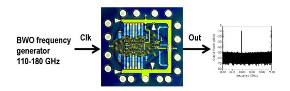
Figure 5.4: 110-136 GHz divider testing
