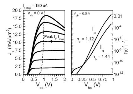
Figure 4.14: Common-emitter I-V and Gummel characteristics, DHBT 25
