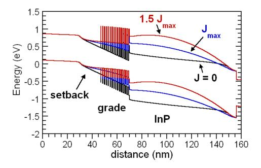
Figure 2.3: Variation of band diagram at  $V_{cb} = 0$ , J = 0,  $J_{max}$ , and 1.5  $J_{max}$
