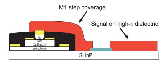
Figure 3.5: Old HBT process after passivation and Metal-1 interconnect
