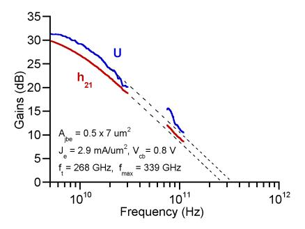
Figure 4.37: Measured microwave gains for 200 nm collector metamorphic DHBT – Peak  $f_{\tau}, f_{max}$
