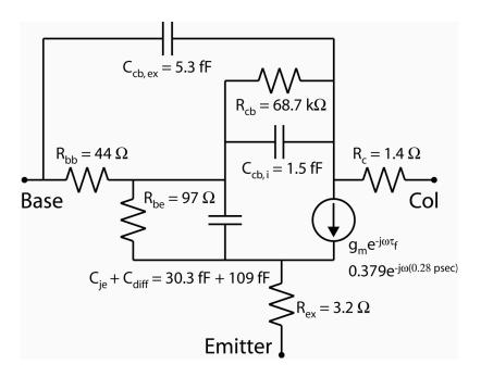
Figure 4.7: Hybrid- $\pi$  model, DHBT 22 – Peak  $f_{\tau}$ ,  $f_{max}$
