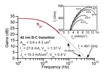
Figure 4.16: Measured microwave gains, DHBT 25 – Peak  $f_{\tau}$
