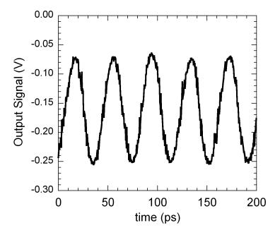
Figure 6.4: Ultra low power CML divide-by-2 output waveform –  $f_{clk,max}$  = 51 GHz,  $f_{out}$  = 25.5 GHz
