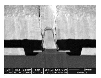
Figure 3.3: Cross-sectional SEM of an HBT after passivation and interconnect metal
