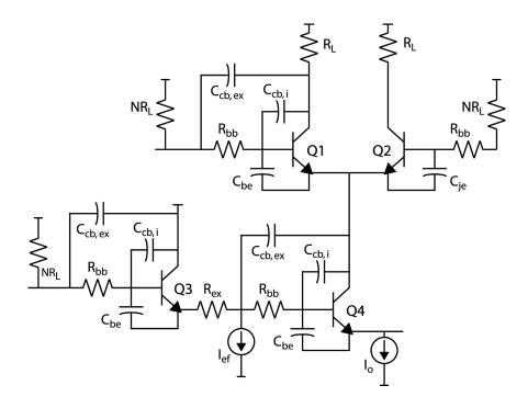
Figure 2.12: Delay path and capacitors charged during clock transition
