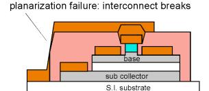
Figure 3.1: Failure mechanisms that limit yield for mesa HBTs
