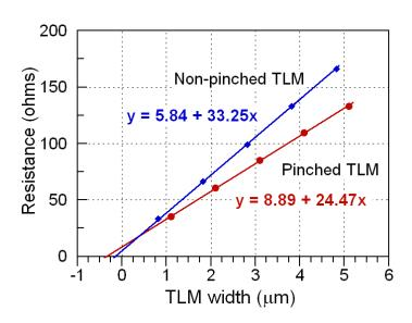
Figure 2.6: Measured TLMs – Pinched and Non-pinched for DHBT 27
