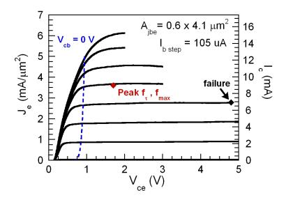
Figure 4.9: Common-emitter I-V characteristics, DHBT 24
