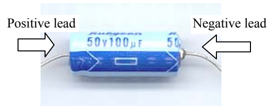
Figure 2-10 – Electrolytic capacitor with axial leads. This particular capacitor is a 100 \mu F with a maximum rated voltage of 50V. The lead on the right is indicated as “negative”.
