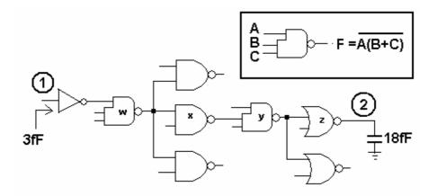
a) A three-input XNORT gate (see insert above) works like a two-input NOR as long as input A is high; otherwise, the output is stuck high. Implement the XNORT gate in complementary CMOS, and size all transistors such that the worst-case delay is equal to that of a minimum sized 2/1 inverter. Find the logical effort associated with each input.
