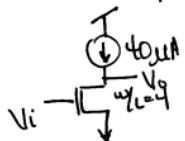
Consider transistor parameters:  $\frac{V_{mox}}{2} = 250 \mu A / \lambda^2$
