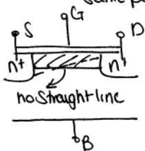
$$V_{TB} = V_{FB} + 2\phi_f + \gamma \sqrt{2\phi_f}$$
