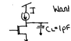
$$\text{pole} = \frac{1}{r_o(C_L + C_{db} + \text{current source})}$$
