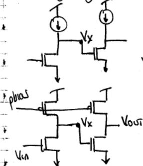
$V_{dd}$  or GND? → No, because one of the devices must be off to allow point to go to  $V_{dd}$  or GND
