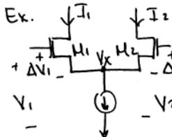
$$V_1 - \Delta V_1 + \Delta V_2 - V_2 = 0$$
