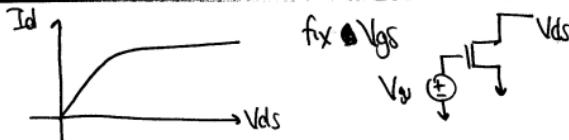
$r_o$  is necessary for the transistor to satisfy physical constraints, without  $r_o$ ,  $g_{m1}$  would be infinite
