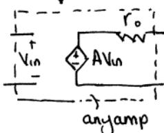
$$\text{pole} = \frac{1}{r_o C_{out}} = \omega = 2\pi f$$
