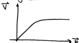
$\vec{V} = \mu \vec{E}$   $\rightarrow$  when field is ~~is~~ small this is valid, relationship is linear
