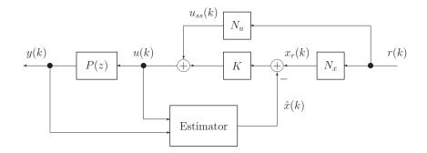
The control is applied using the estimated state,  $\hat{x}(k)$ , in place of the true state, x(k).
