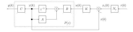
Design the state feedback gain, K, for good closed-loop pole positions.
