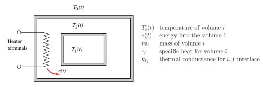
We can derive the state-space representation directly from the thermal energy equations.
