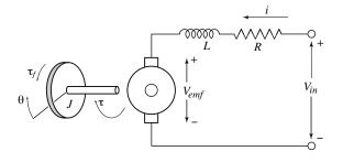
The "back emf" is proportional to motor speed:  $V_{emf} = K \frac{d\theta}{dt}$ .
