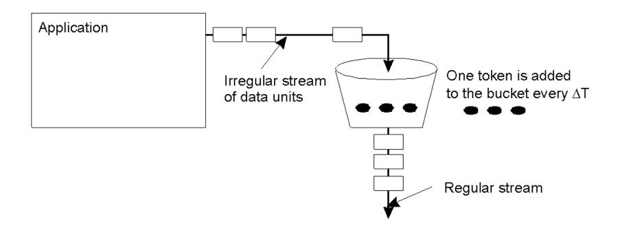
The principle of a token bucket algorithm.
