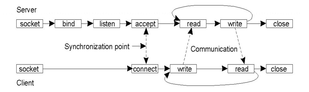
Connection-oriented communication pattern using sockets.
