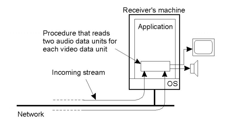
The principle of explicit synchronization on the level data units.
