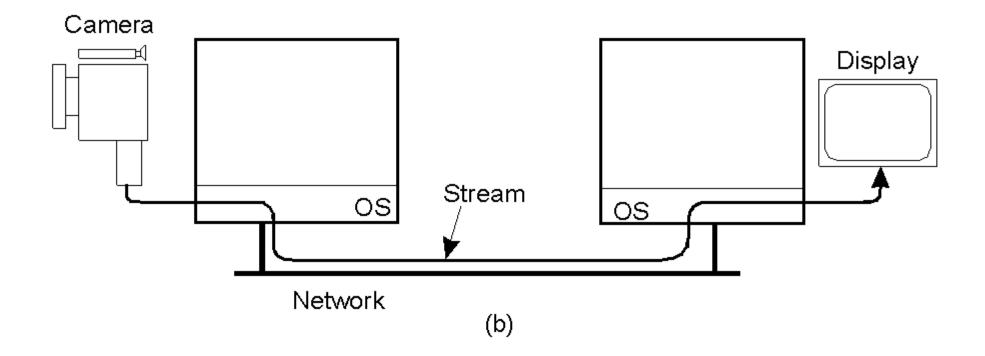
Setting up a stream directly between two devices.
