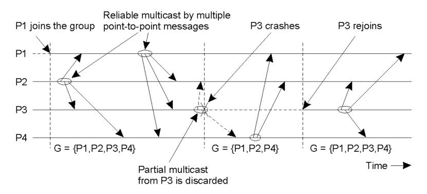
The principle of virtual synchronous multicast.
