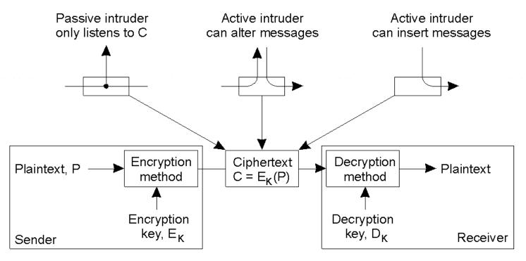
**Symmetric system:** Use a single key to encrypt the plaintext and decrypt the ciphertext. Requires that sender and receiver **share** the secret key.
