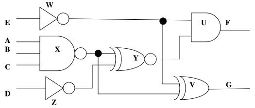
In this problem, the letters U,V,W,X,Y,Z label gates; A, B, C, D, E are inputs, and F and G are outputs.
