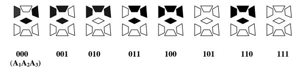
Design a digital circuit that takes the input from the counter and displays the correct output pattern on the 7-segment display. Your circuit should use only 2-, 3-, and 4-input NOR gates and inverters. Try to minimize the number of gates required. Any solution which uses 11 or fewer gates (not counting the four inverters for the inputs) is acceptable.
