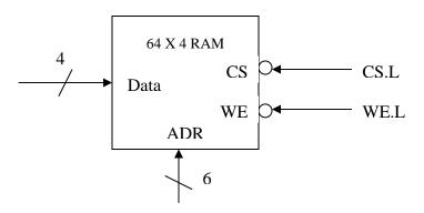
(**30 points**) (c) Assume that the SPR has already received the first 16 bits of a 256-bit packet. Draw a timing diagram which shows ALL the relevant control signals necessary for writing in the next 8 bits of the 256-bit packet, and updating the RAM address. Assume that the control signals are generated by a Moore-type finite state machine running at 4 MHz. Show as many signals as necessary.
