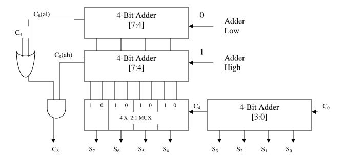
Figure: 8-bit carry select adder
