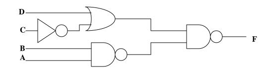
Find a simple expression for F by pushing the bubbles from the output towards the input variables, step by step. Write down a simplified expression for F at the end.
