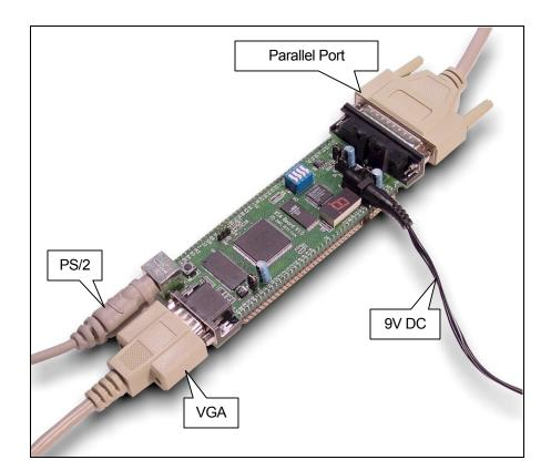
• Figure 1: External connections to the XSA Board.
