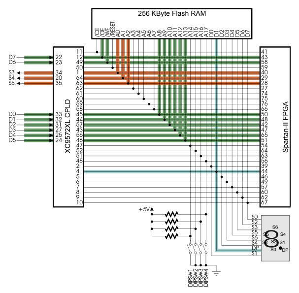
receiving data from the FPGA over the status lines. The connections between the FPGA and the parallel port are shown below.
