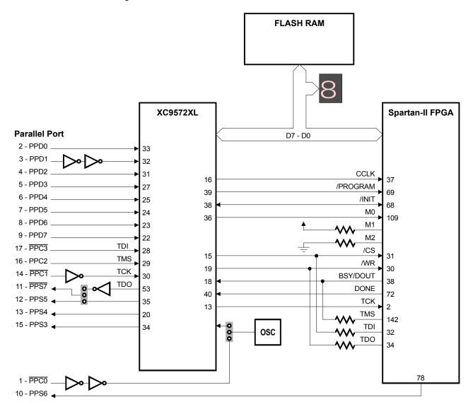
After the SpartanII FPGA is configured with a bitstream and the DONE pin goes high, the CPLD switches into a mode that connects the parallel port data and status pins to the FPGA. This lets you pass data to the FPGA over the parallel port data lines while
